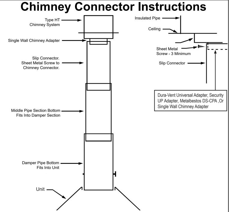
The above illustration represents the installation procedure for dripless pipe installation. This installation method of installing the connector pipe with the male end down allows for any moisture to remain on the inside of the connector pipe.
