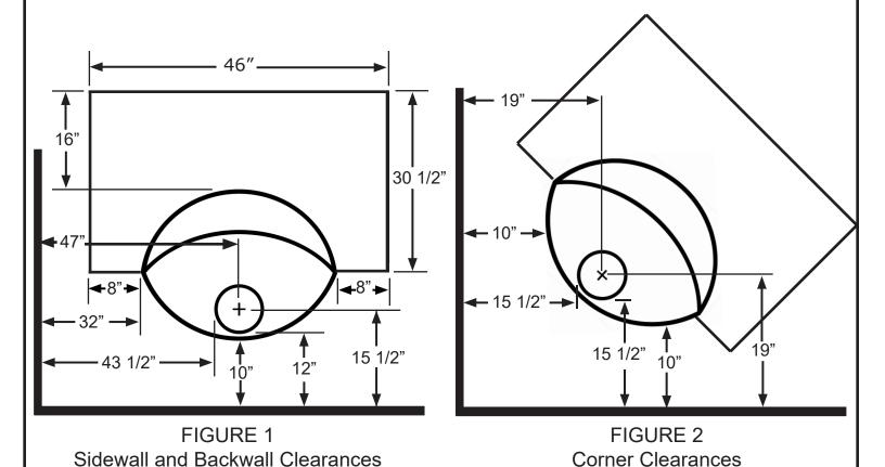
Hearth dimensions shown are minimum requirements. It may be desired to exceede these minimum dimensions for a more decorative installation. The hearth material must be 3/8" or thicker noncombustible material. It is not required for the hearth material to extend under the base of the fireplace.
